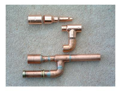
The venturi is assembled from readily available plumbing fittings, and the photograph above shows both a complete assembly, and most of the component parts laid out alongside.
